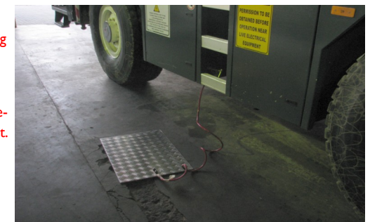
Above: 55ton LTM1060 Liebherr - Eskom in process of earthing connections.
